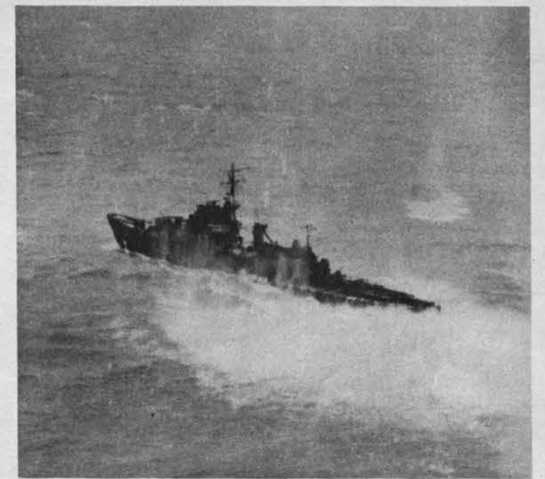
Kaibokan 2 hull has a flat taper aft to squarish stern. Depth charge equipment is prominent aft. Kaibokan is Jap word for escort vessel.
